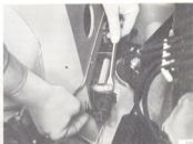
Location of camber adjustment spacers
