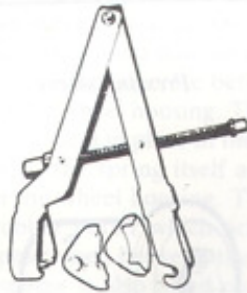
85 95 839 (A3) Spring compression tool for removal and fitting of front coil spring
