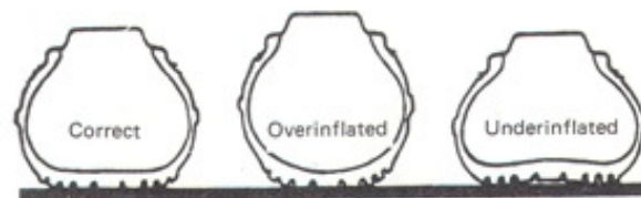
Contact between the tyre and the road
