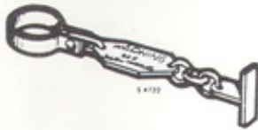
89 96 076 (A3) Safety chain for spring shanks
