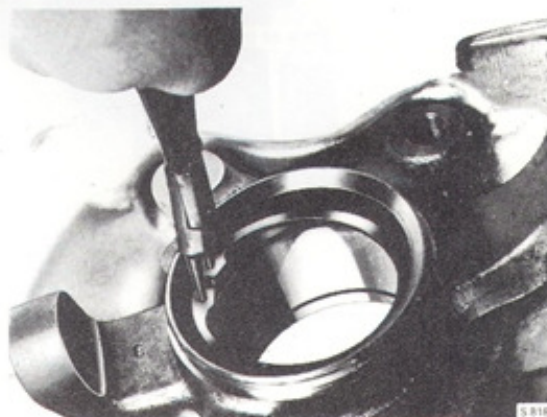
Pressing out the bearing (outer race)
