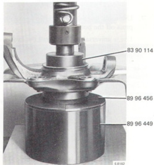
Pressing out the bearing (outer race)
