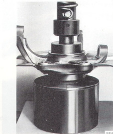
Pressing out the bearing (outer race)
