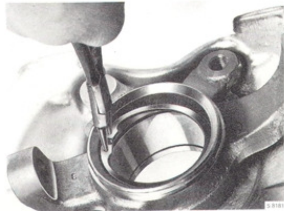
Removing the circlips
