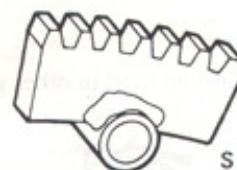
83 92 987 (A1) Locking segment for locking of crankshaft
