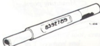
83 92 789 (A2) Drift installation of fuel jet, carburetor
