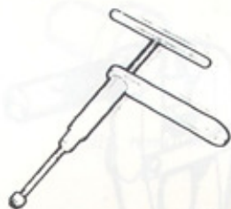
83 93 035 (A0-1) Adjusting tool, fuel needle
