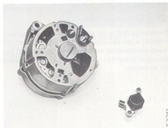
The voltage regulator removed from the alternator
