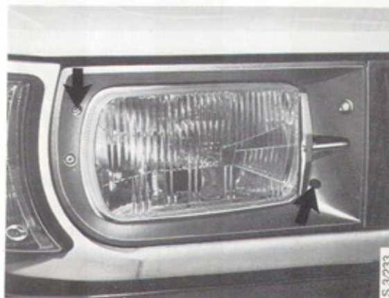
Headlight adjusting screws
