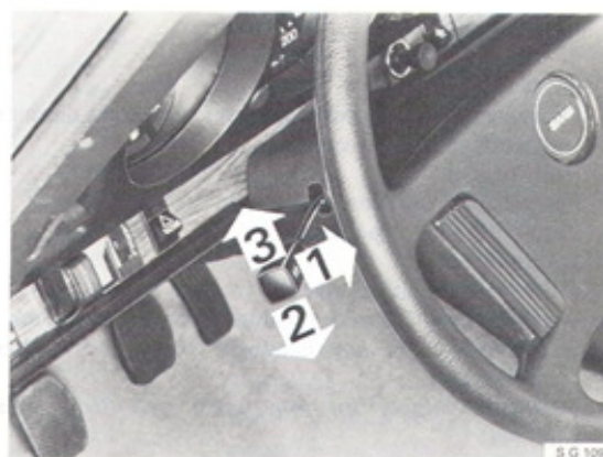
Direction indicator, headlight flasher and dimmer switch
