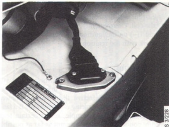
Distributor with Hall transmitter
