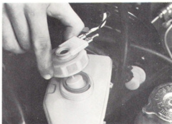
Brake warning light switch
