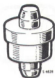
83 91 997 (A2) Drift for clutch shaft seal (transmissions with chain-drive primary gear), needle bearing in primary gear housing
