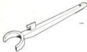
83 93 175 (A1) Lever for removal of clutch shaft (also suitable for fitting of spacer ring)
